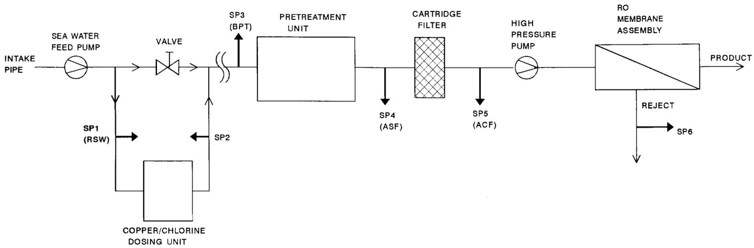
Fig.4 Layout of SWCC experimental Reverse Osmosis (SWRO) pilot plant, showing Sampling Points (SP). See text for legend
